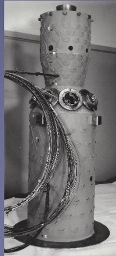
**Mini 6- inch diameter prototype Low NOx
