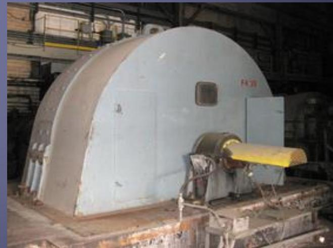
GE 5000 HP DC Motor in steel mill driving stainless strips across rollers
